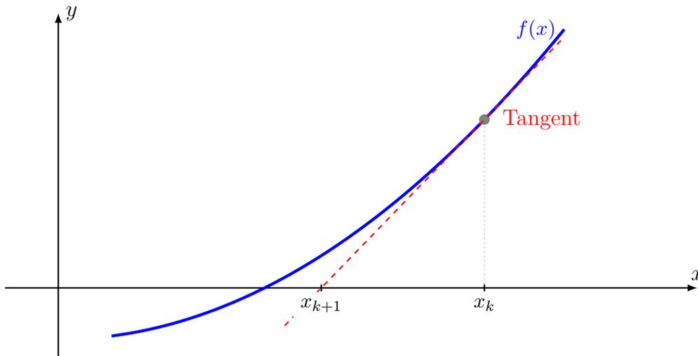
Figure 5.2: Graphical illustration of a Newton–Raphson iteration. The code used to create this figure is based on the answer <https://tex.stackexchange.com/a/551205/125558> on L<sup>A</sup>T<sub>E</sub>X stack exchange.
