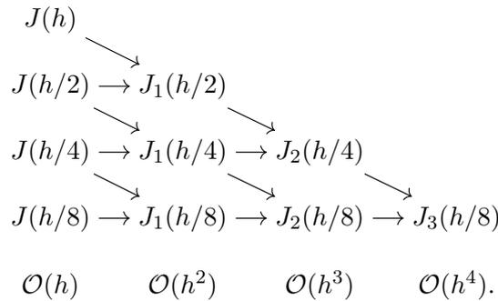
Here, the last row indicates the scaling of the error with respect to the parameter  $h$  in the limit as  $h \rightarrow 0$ . The linear combination in order to calculate  $J_i(h/2^i)$  is always of the form
